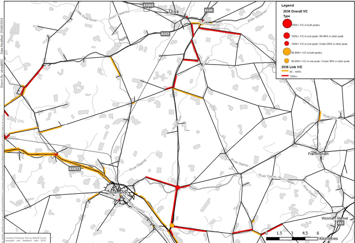
**Figure 22 – A140 Corridor – 2036 Links and Junctions with V/C 85%+**
