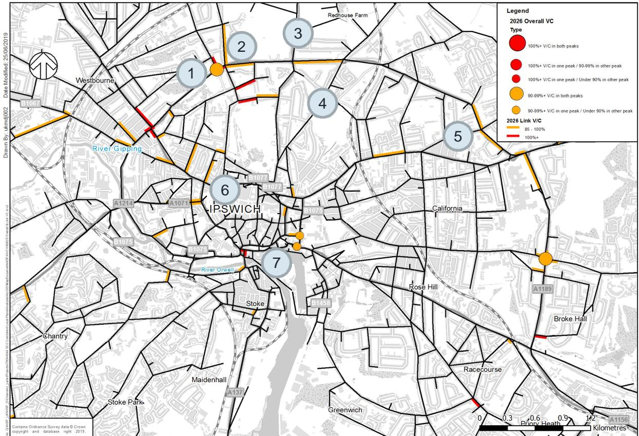
3.9.4. Figure 16 shows the overall junction V/C and link-based V/C above 85% within Ipswich in 2036.
