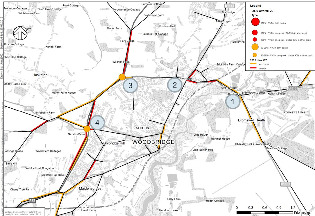
3.8.9. The 2036 modelling results with the demand reduction show that despite the demand reductions which have been applied the Melton Crossroads junction continues to have approaches which are over capacity, consistent with previous results reports. The southern Melton Road arm does show improvement in the PM peak, reducing from 86% V/C in the previous Jan 2019 modelling to 63% V/C in the modelling with demand adjustments.
