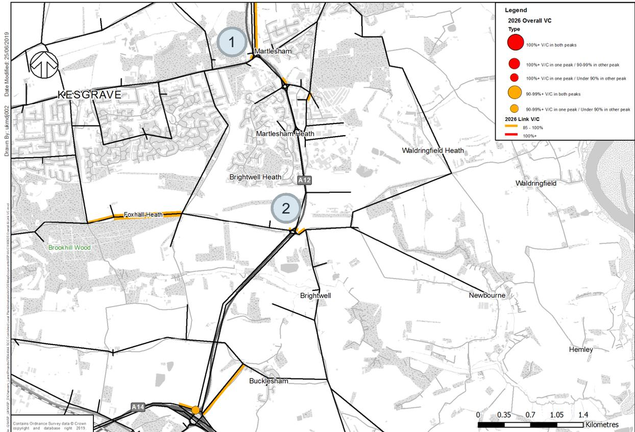
3.8.12. Figure 10 shows the V/C performance around the A12 East of Ipswich corridor for 2036. The following junction approaches are shown to be over capacity:
