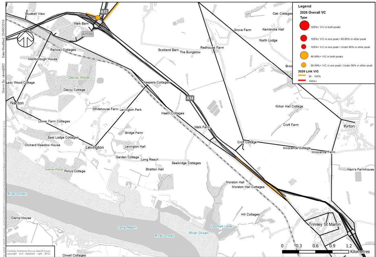
3.8.20. Figure 14 shows the links which are over capacity or close to capacity in 2036. The Street in Nacton is over capacity as a result of congestion on the westbound on-slip at the Nacton Interchange (A14 Junction 57). As a result of this delay traffic opts to re-route away from Ipswich Road / Nacton Road in order to access the A1156 Felixstowe Road.
