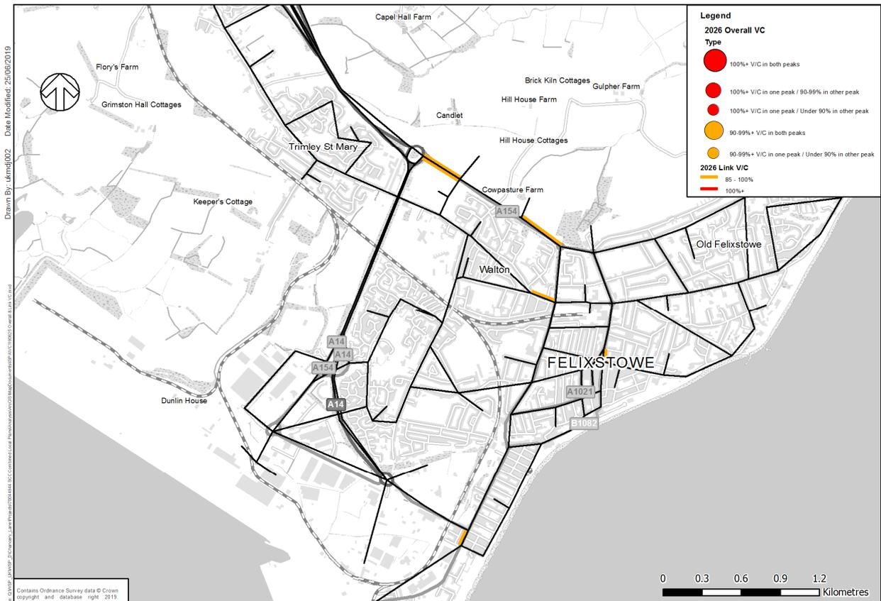
3.8.16. Figure 12 shows the over-capacity and close to capacity links within Felixstowe in 2036.
