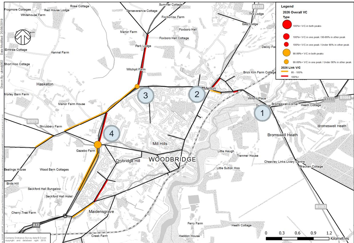
3.8.8. Figure 8 presents the overall junction and link-based V/C for both Woodbridge and Melton in 2036
