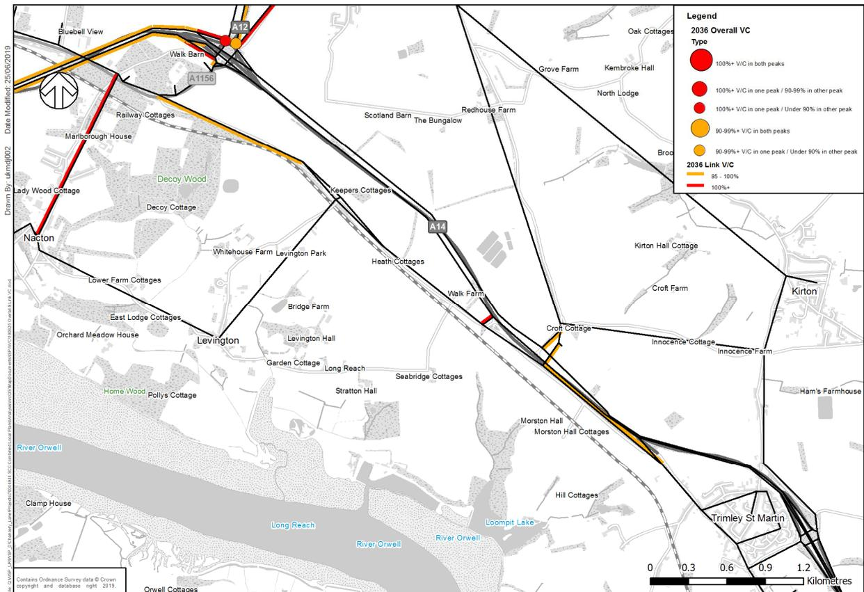
3.8.21. The 2036 modelling results with the demand reduction show a similar pattern level of capacity issues compared to the previous January 2019 report. The main differences are that Innocence Lane is no longer shown as being over capacity on the approach to the left-in / left-out junction onto the A14, and the eastbound route parallel to the A14 to Trimley St. Martin is no longer over capacity. These differences occur because the demand adjustments lessen the cumulative impact.
