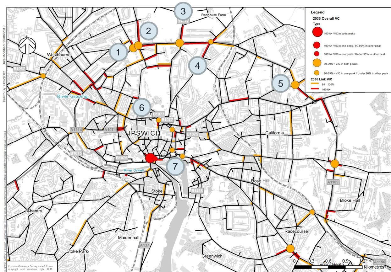
3.9.5. The 2036 modelling results with the demand reduction demonstrate that a total of five junctions (as per Table 17) are no longer flagged as having V/C issues. However, numerous junctions around the A1214 are shown to have capacity issues as per the previous results report. However, the latest modelling shows a fewer number of links which are over capacity compared to the previous modelling.
