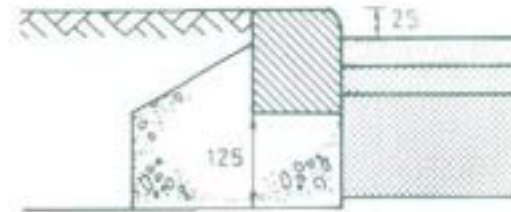
127 x 150 Kerb used for Mews Court and alternative for Shared Surface Roads
