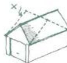
Avoid pitching roof wrong way when freestanding.
